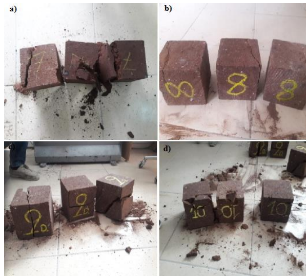
Fig. 7. Ahlat Stone Samples Broken after Combined Curing
