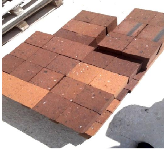
Fig. 2. The Appearance of Natural Ahlat Stone after Cutting
