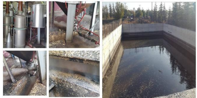
Figure 1. Discharge of waste rose petals and wastewater to the drainage channel and lagoon (Başbuğ Çancı, 2017).
