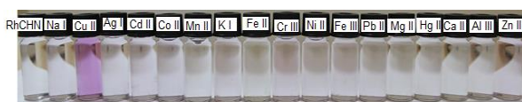
Figure 3. The color change of RhCHN after addition of each competitive metal ions (2.0 equiv) in buffer solution.
