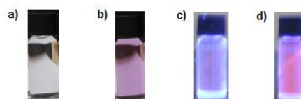
Figure 5. The picture shows the color change of free RhCHN (a); and after addition of 2.0 equiv. of Cu 2+ (b); under natural light; (c) and (d) the fluorescence image of the same solutions (a & b) excited by UV lamp ( \lambda_{\text{ex}} = 365 nm) in buffer solution.
