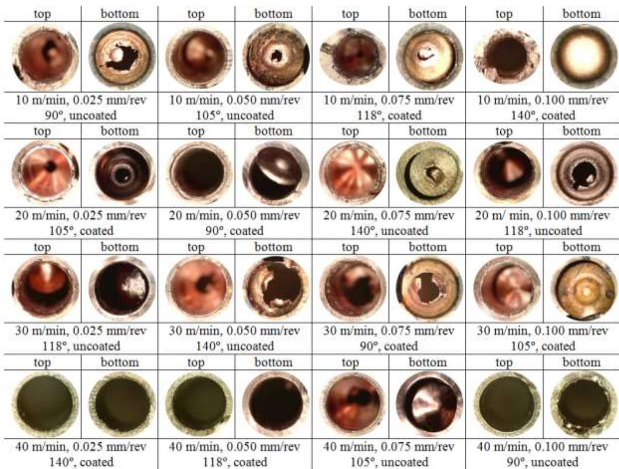
Figure 6. Top and bottom views of holes (entrance and exiting of the holes)
