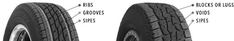
Figure 5. The pattern of tire print [15]
