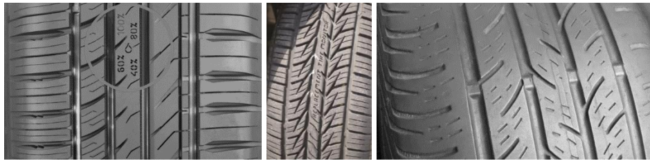
Figure 2. Tire treadwear indicators [13, 14]
