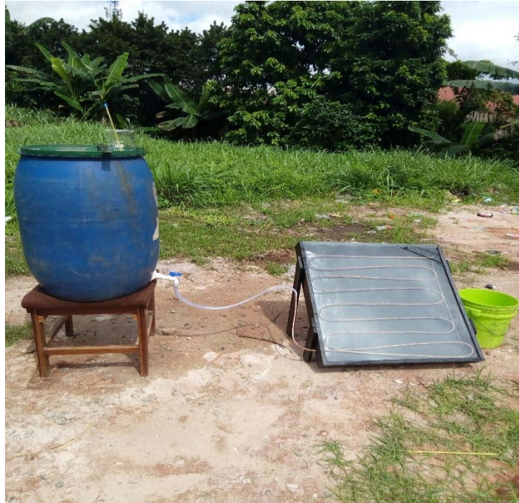
Figure 1. Experimental setup of the flat plate solar collector
