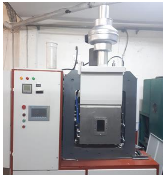
Figure 1. PLC controlled direct hot pressing machine.
