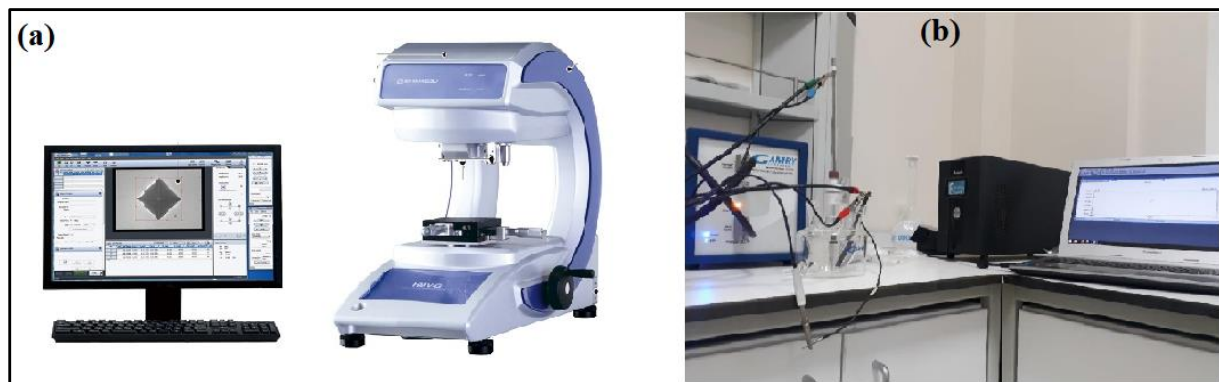
Figure 3. (a) SHIMADZU HMV-G21 model microhardness measuring device, (b) Reference 3000 Potentiostat / Galvanostat / ZRA device.
