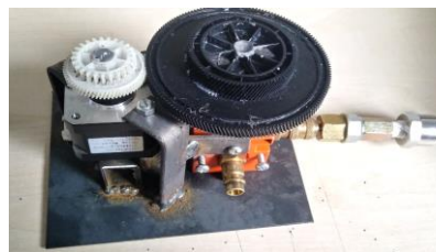
Fig. 4. Stepper motor pressure sensor connection for simulation pressure
