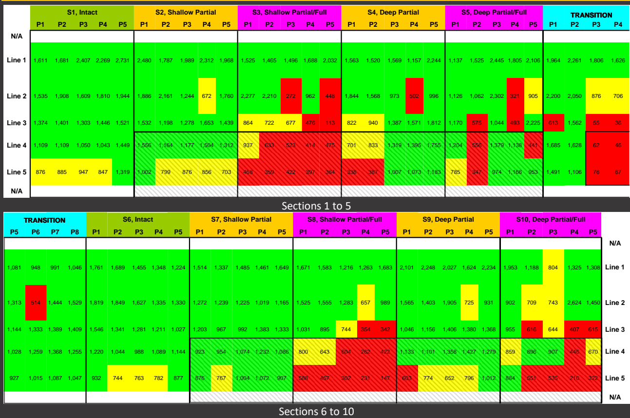
Figure 7. Temperature-Adjusted Contour Maps of FWD Moduli in Cool Weather based on Revised Statistical Criteria
