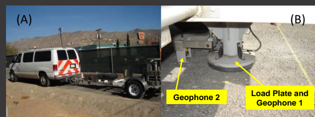
Figure 1. Falling Weight Deflectometer on Small Scale Study; (A) FWD, (B) Loading Plate
