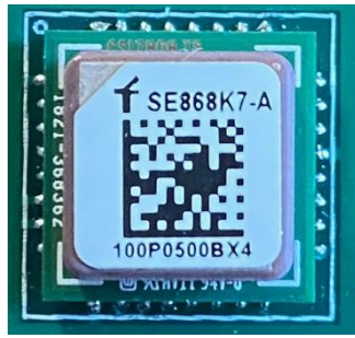
Figure 4- GPS module for tracking global position of the tractor
