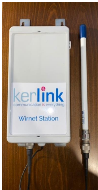
Figure 5- LoRaWAN gateway for data transmission
