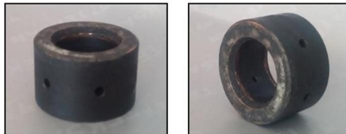
(c) Appearance of Turbo Bearings after 1500 hours of operation
