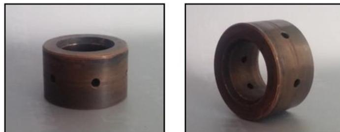
(b) Appearance of Turbo Bearings after 750 hours of operation
