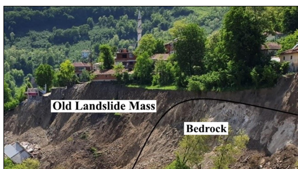
Figure 12: Crown area of main scarp cut partly an old landslide mass and partly the bedrock and debris cover on it.
