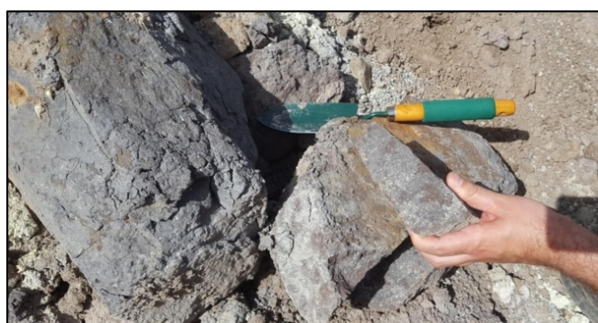
Figure 11: Andesitic bedrock pieces come out in the eastern part of the crown area of main scarp and partially altered.
