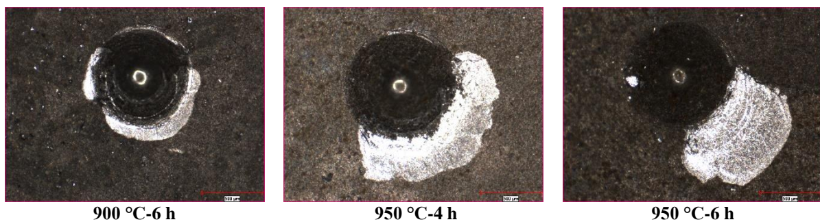
Figure 6. Boride layer removals occurring after the adhesion test in AISI 304L samples pack-borided with microwave hybrid heating
