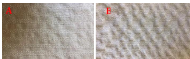
Figure 8. A) Appearance of Sample 4 before heat treatment, B) Appearance of Sample 4 after heat treatment [2].
