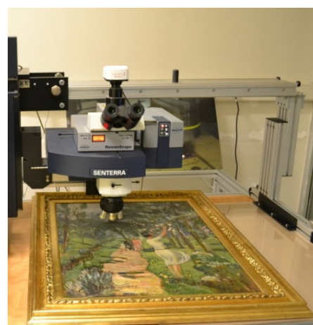
Figure 1. The raman spectrometer, which was used in this study, equipped with a confocal microscope mounted onto a crane.
