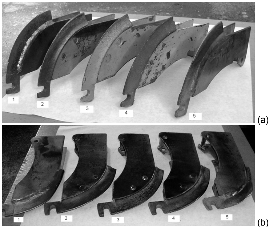
Figure 2. Appearances of unworn (a) and worn (b) drill cultures used in this research. (1. C 1050 (C45), 2. 27 chromium (G-X 300 CrMo), 3-4. Ni-hard 4/1 and 2 (G-X 300 CrNiSi), 5. Citadur 600 B)
