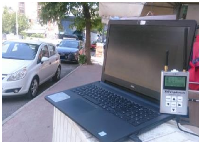
Fig. 2. An example of spectrum measurement with spectrum analyzer
