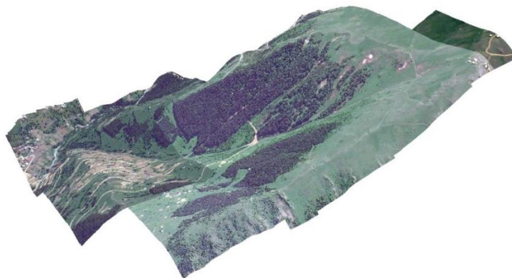
Figure 4. DEM (5 m pixel resolution) overlapped with aerial photo
