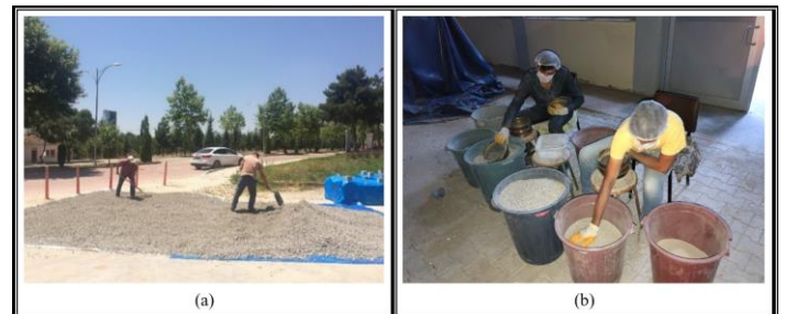
Figure 5. Pumice aggregates to be used in HPLC production: a) Drying of pumice aggregates for sieve analysis, b) Pumice aggregates remaining on each sieve in accordance with TS EN 933-1.
