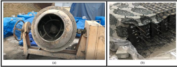
Figure 6. Production of high performance lightweight concrete: a) Concrete mixer, b) Curing application of Belgium Hinged Beam test samples.
