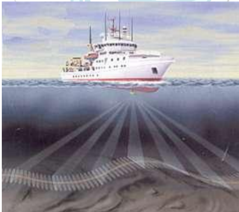
Figure 4. Hydrographic Surveying by Research Ship
