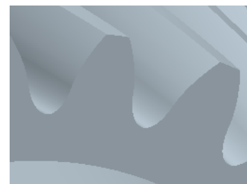
(b) Helical gears with single circular fillet curves
