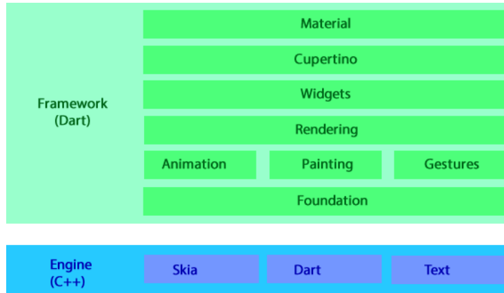
Figure 2. Flutter's structural framework (Architecture, 2020)
