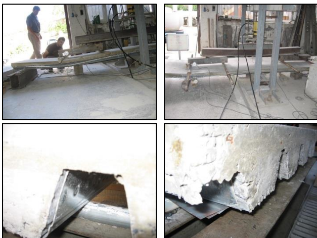
Figure 11 Testing of double span bending tests
