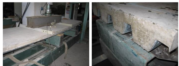
Figure 9 Testing of single span bending tests
