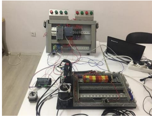
Figure 4. S7-1200 PLC connected system
