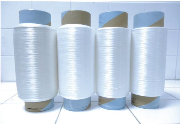
Figure 4. Produced PP filament yarns in this study [6]
