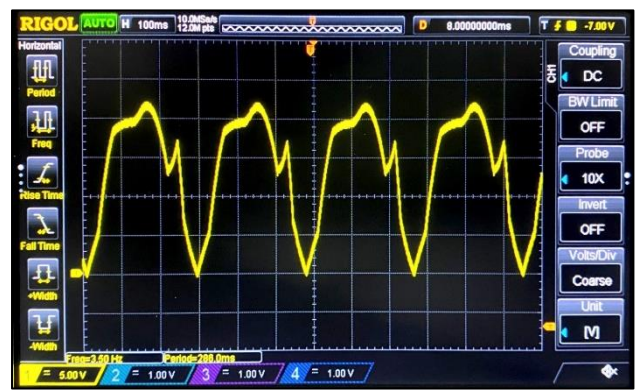
Figure 20. Ventricular Tachycardia observed on oscilloscope
