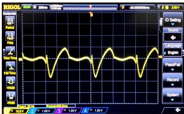
Figure 21. Ventricular Paced observed on oscilloscope
