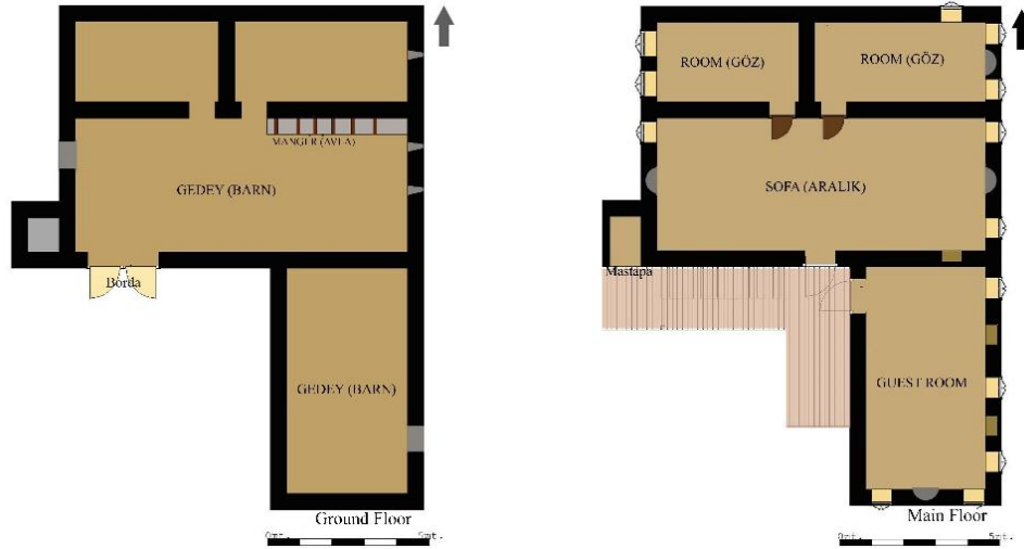
Figure 10. Schematic Plan of Ground and Main Floors
