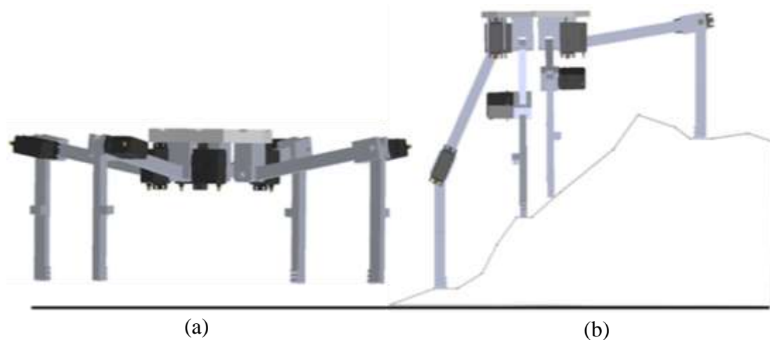
Figure 3. Position of the landing gear on level ground (a) and on sloping ground (b).
