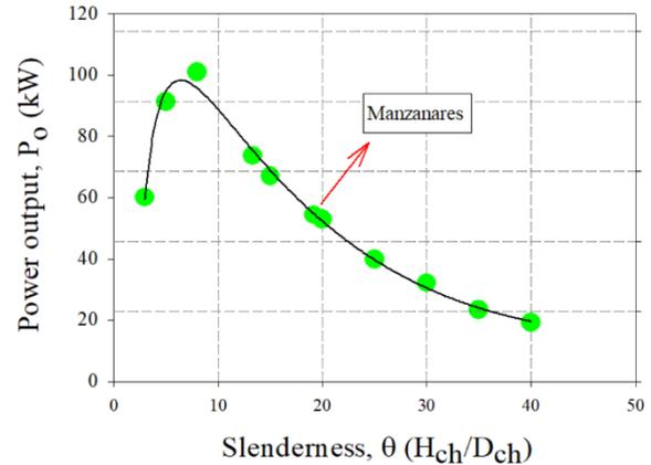
Figure 8. Effect of slenderness on power output
