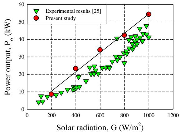
Figure 3. Verification of the CFD model via the power output ( $P_o$ )
