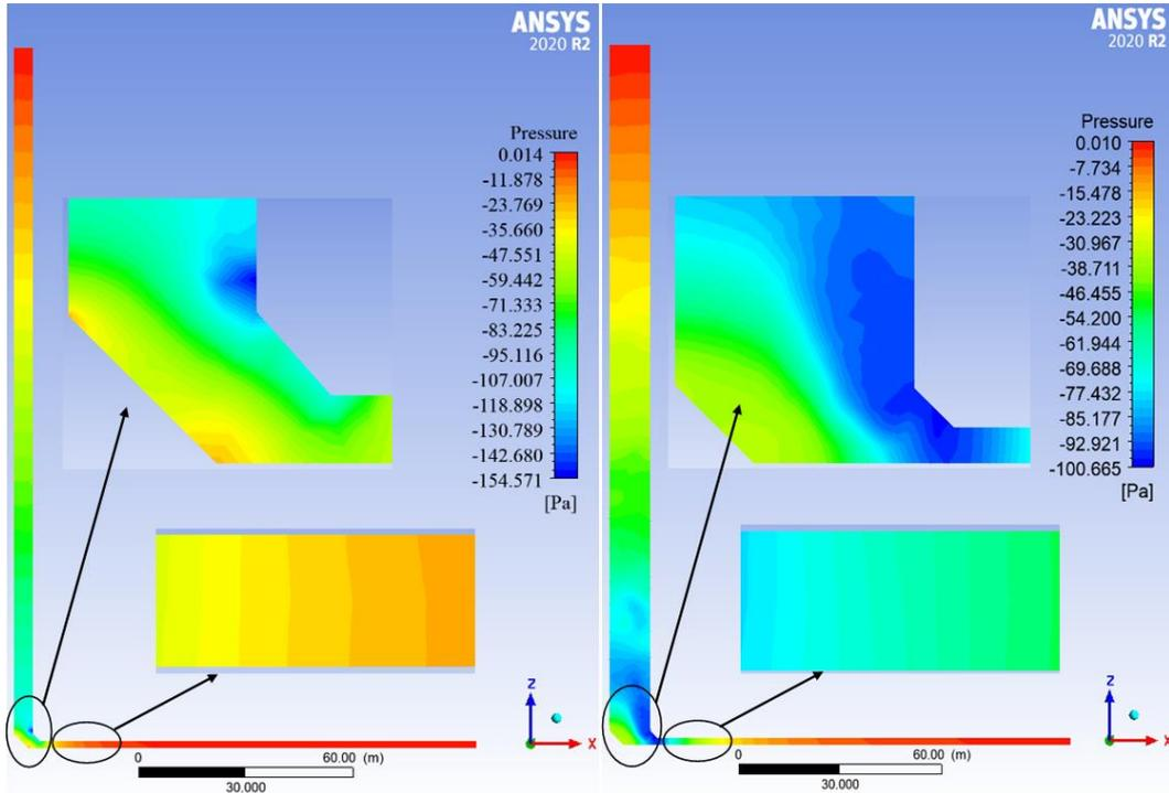
Figure 4. Pressure distributions for reference geometry and  $\theta=8$
