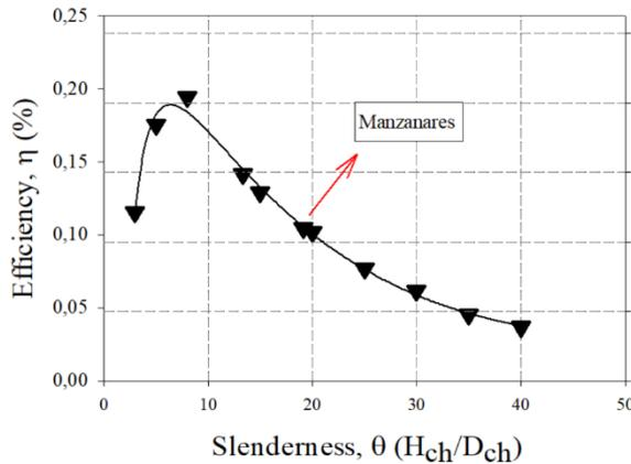
Figure 9. Effect of slenderness on system efficiency
