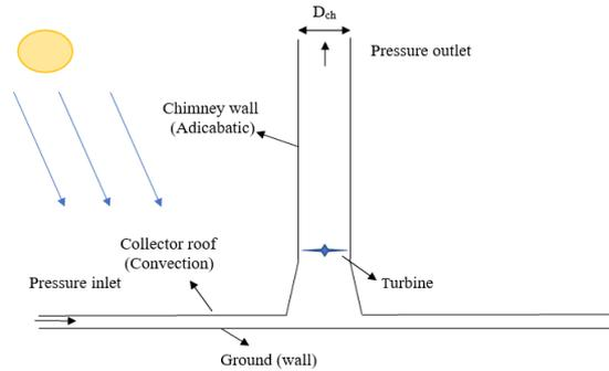
**Figure 1.** The model for SCPP system and relevant boundary conditions(*SCPP sistem modeli ve ilgili sınır koşulları*)
