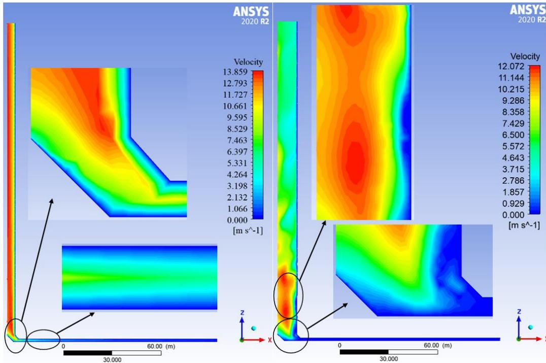
Figure 5. Velocity distributions for reference geometry and  $\theta=8$
