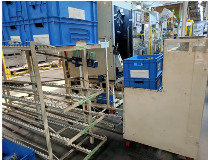
Figure 9. Karakuri and racking system integration
