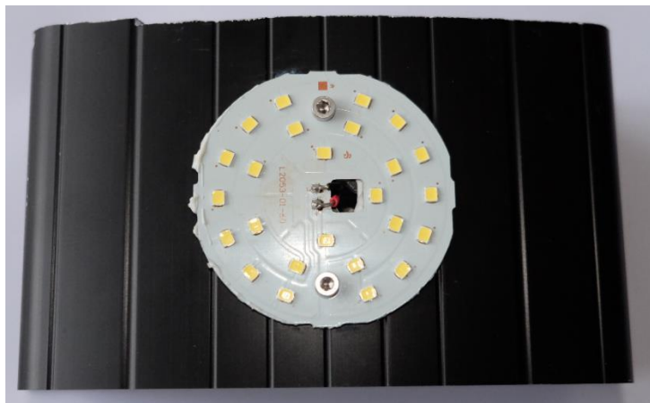
Figure 7. Transmitter design with aluminum enclosure
