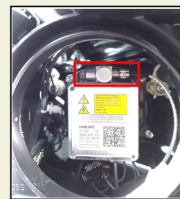
Figure 6. Rotational accelerometer placed on the rear side of light module
