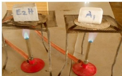
Figure 3. Experimental set-up of the flame resistance test on the composites.
