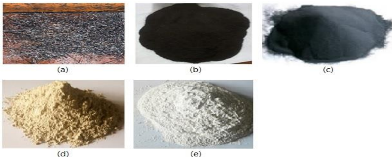
Figure 1. Input materials used for the study (a) mild steel chips (b) 105- \mu\text{m} ground and sieved mild steel particles (c) As-received 53- \mu\text{m} silicon carbide (d) As-received 90- \mu\text{m} bentonite (e) As-received 90- \mu\text{m} magnesia.
