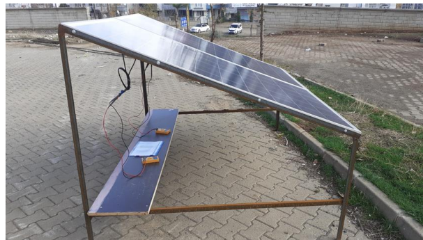
Figure 3. Measurement of short circuit current and open circuit voltage
