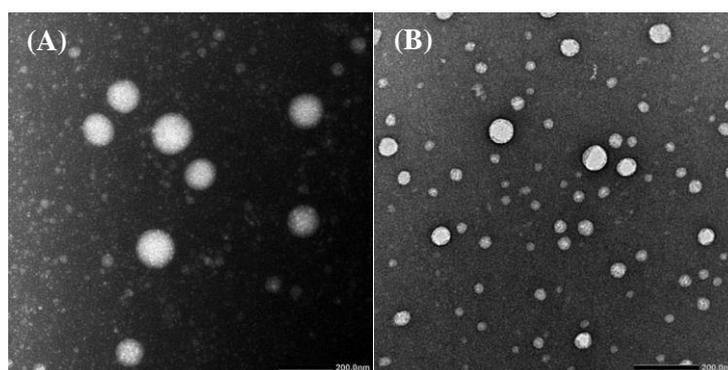
Figure 4. Transmission electron micrograph of cinnamon NE (A) and cinnamaldehyde NE (B). The TEM was performed on a JEOL JEM-1400 Plus transmission electron microscope operating at an acceleration voltage of 80.0 kV with a 20 mm aperture. Print magnification 30000x.
