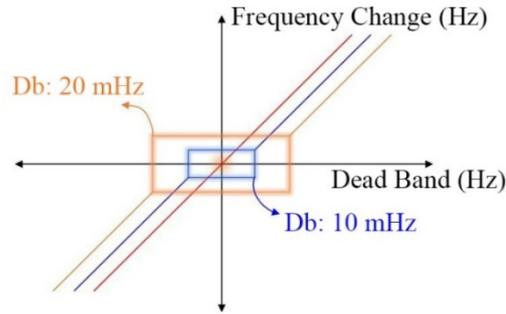
Figure 7. The response characteristic of the BESS for PFC
