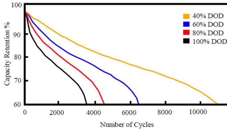
**Figure 3.** Capacity retention according to number of cycles
