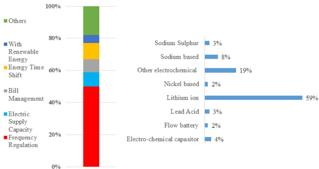
**Figure 2.** The main usage services of electrochemical energy storage
