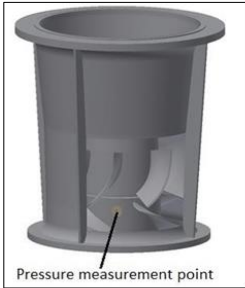
Figure 8b. Pressure measurement location (piezoelectric pressure transducer)
