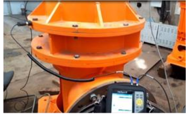
Figure 10. Measuring with Vibxpect II analyzer
