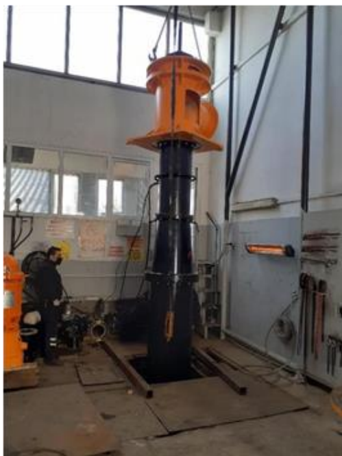
Figure 9b. Placing the pump to the test bed
