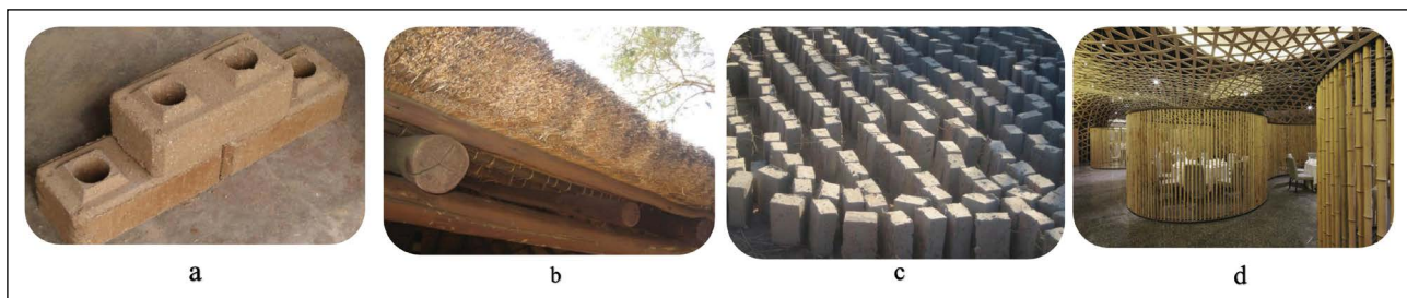
Figure 1. (a) stabilized interlocking bricks, (b) straw (thatch), (c) Adobe, (d) Bamboo. Source: [7, 8].
