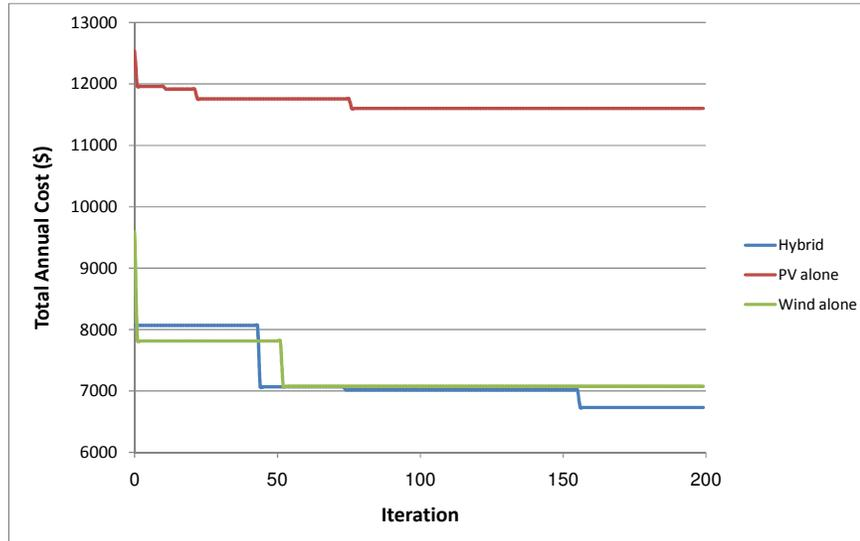
**Figure 6:** Convergence process of ACO for finding the optimum size of the systems (case study 1)
