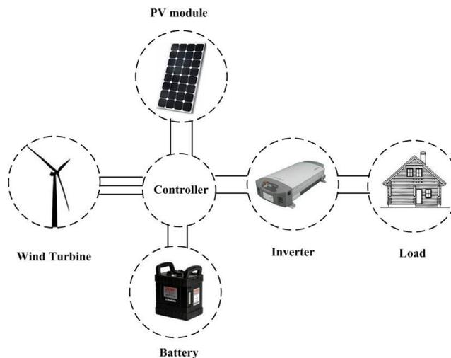
**Figure 1:** Representation of PV/wind/battery hybrid system
