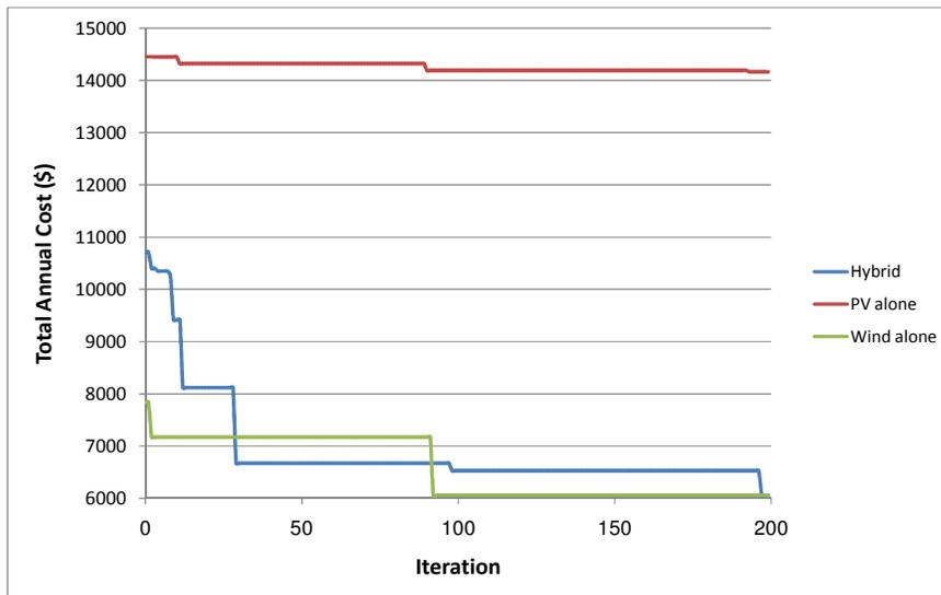
Figure 7: Convergence process of ACO for finding the optimum size of the systems (case study 2)
