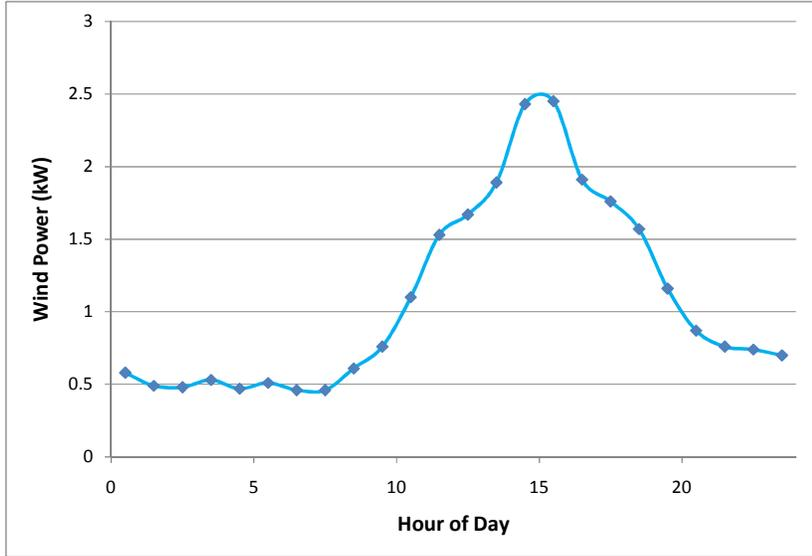
**Figure 4:** Average hourly power generated by a wind turbine in a day
