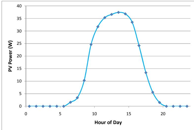
Figure 3: Average hourly power generated by a PV panel in a day
