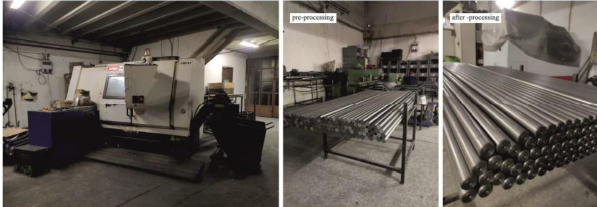
Picture 2. CNC lathe - raw material - lathed product
