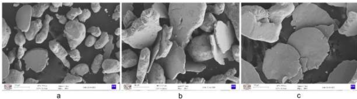
Figure 7. SEM images of ground AA7075 powders: 5:1 ball to powder ratio-30 min (a), 10:1 ball to powder ratio-60 min (b) and 20:1 ball to powder ratio-90 min (c).
