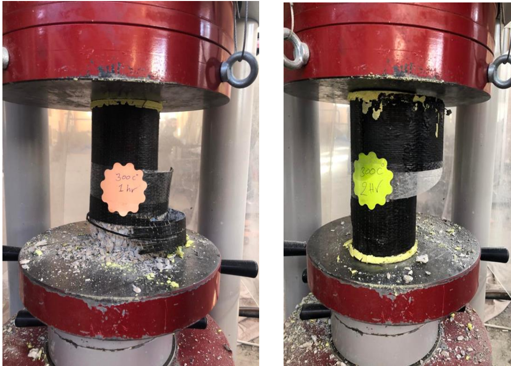
Figure 1. Failure of BFRP wrapped specimens.
