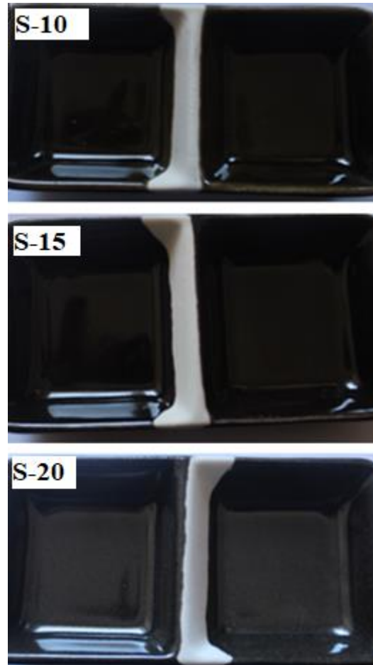
Figure 1. Color effects of 10%, 15% and 20% non-calcinated colorants addition on stoneware glaze, respectively
