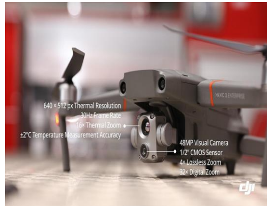
Fig. 2 Properties of thermal drone camera
