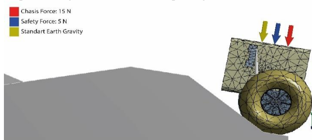
Figure 5. Structural analysis with static loads
