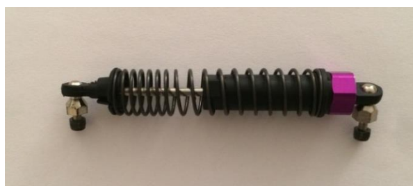
Figure 3. Selected dashpot for robot suspension system
