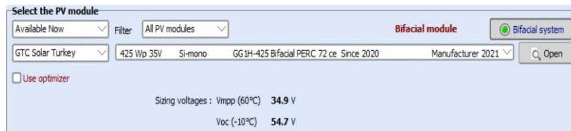
Figure 13. Selecting the PV module.
