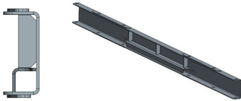
Fig. 8 Left, Bumper Cross Section. Right, Bumper
