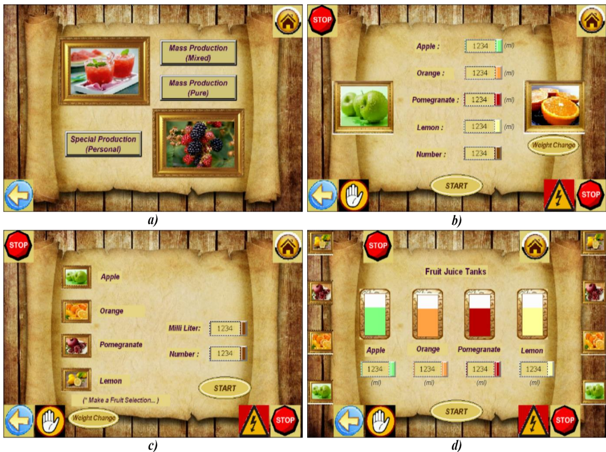
Fig. 8. HMI page designs a) production method selection b) mass production (mixed) c) mass production (pure) d) special production (personal) [25]
