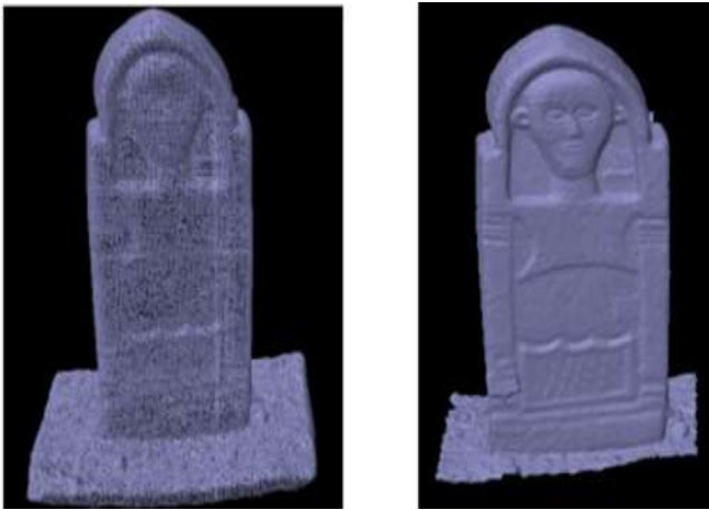
Figure 7. Solid model and tiled triangular model created in Agisoft software for the tomb stele.
