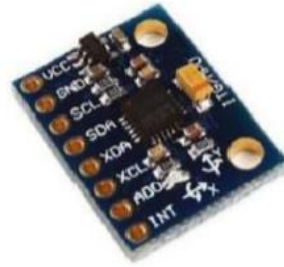
Figure 1. MPU6050 IMU sensor
